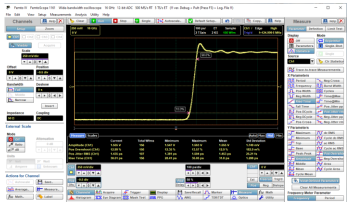
Figure 6. Transient response of the FemtoScope 1161 tested with 1.6 V step having 25 ps rise time. Response shows 31.8 ps rise time and 1.45 ps rms jitter.
