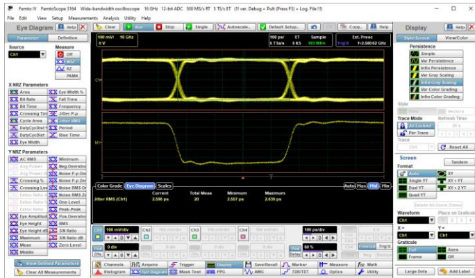
Figure 21. The FemtoScope 3164 used Pattern Lock trigger to generate pattern trigger from 2.5 GHz clock. Eye RMS Jitter = 2.64 ps.
