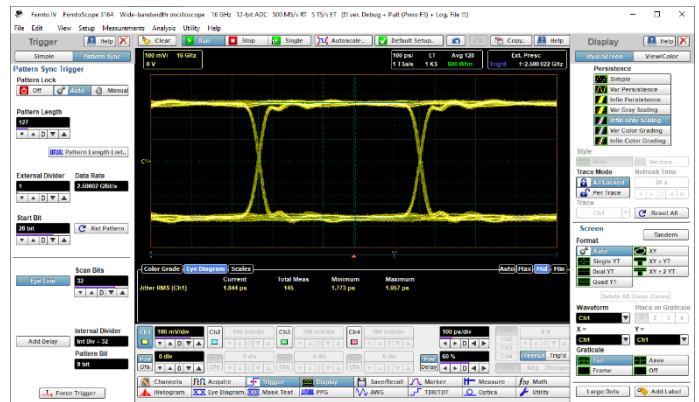
Figure 22. FemtoScope 3164 demonstrates the same average 2.5 Gb/s eye diagram by using Eye Line mode. Eye RMS Jitter = 1.96 ps. Clearly noticeable influence of data dependent jitter.
