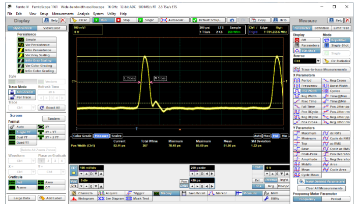
Figure 19. The FemtoScope 1161 demonstrates internal direct trigger from 81-ps pulse having 400 mV amplitude and 781 MHz frequency
