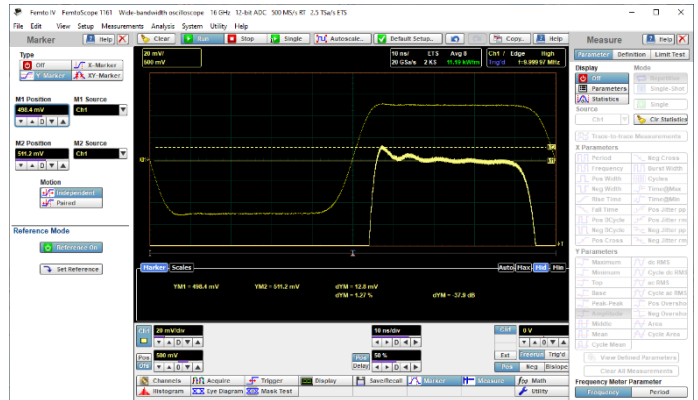
Figure 27. Ratiometric measurements. 1-V pulse is used as a reference. Two Y-markers measure 1.27% peak-peak ringing on the top of pulse.
