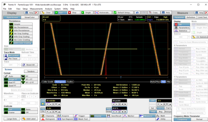
Figure 17. The FemtoScope 1051 surely triggers from 2.5 GHz sinewave with 1.62 ps rms jitter using internal trigger source
