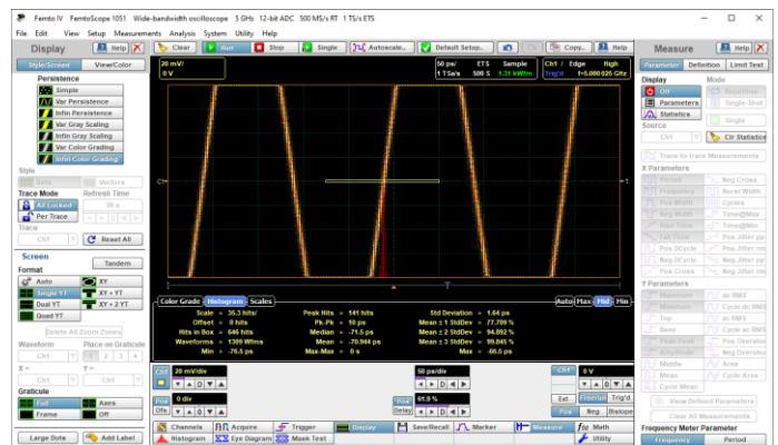
Figure 32. Horizontal histogram measures 1.64 ps rms jitter of 5-GHz sinewave (Std Deviation value).
