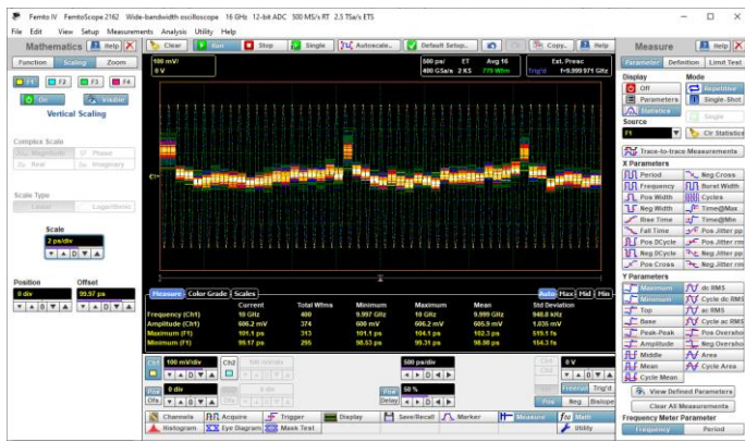
Figure 40. Trend of period measures nonlinearity of oscilloscope time base with 10-GHz sinewave. Maximum trend of period = 102.3 ps. Minimum trend of period = 98.98 ps. Peak-peak nonlinearity is within \pm 2.3 ps at 5 ns timing window.
