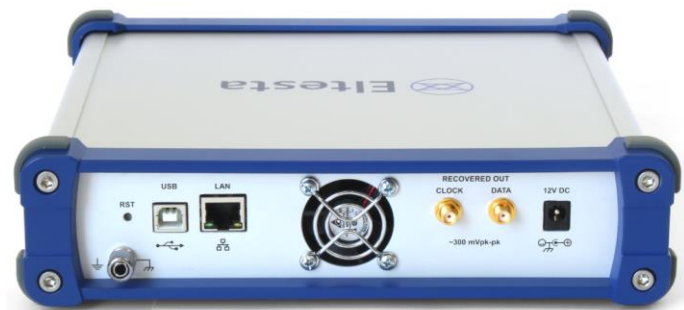
Figure 44. Rear panel of the Femtoscope 3000 with USB and LAN connectors.
