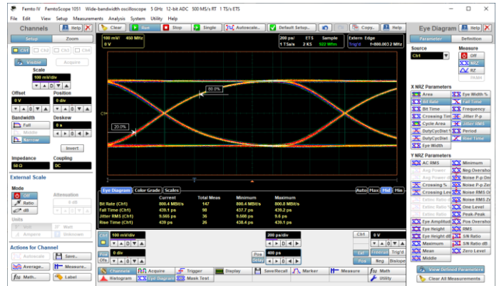
Figure 10. 800 Mb/s wide opened eye diagram acquired in narrow bandwidth mode with the FemtoScope 1051 shows good response characteristics.
