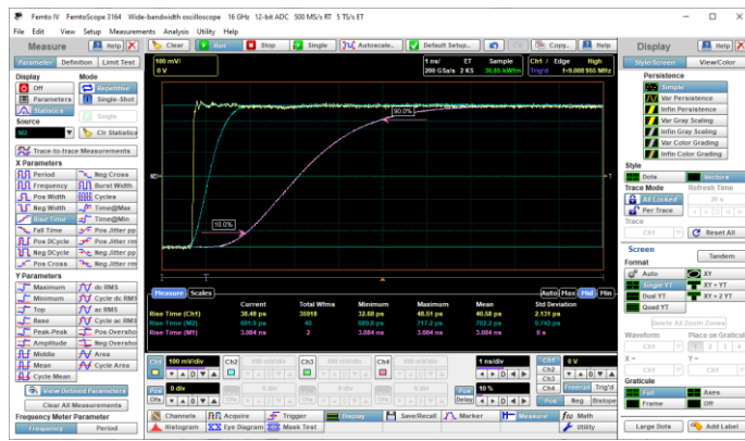
Figure 7. Comparative transient response of the FemtoScope 3164 made for three different bandwidths. Yellow shows 40.58 ps rise time acquired in full 16-GHz bandwidth, blue shows 702 ps rise time acquired in 500-MHz bandwidth and violet shows 3.084 ns rise time acquired in 100-MHz bandwidth.
