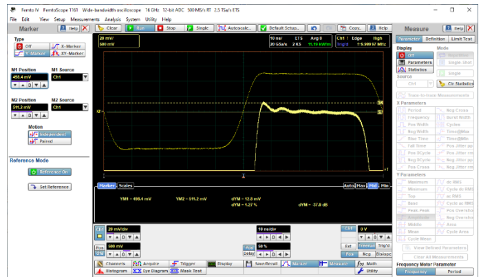
Figure 27. Ratimetric measurements. 1-V pulse is used as a reference. Two Y-markers measure 1.27% peak-peak ringing on the top of pulse.
