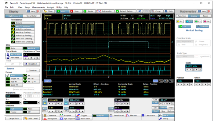
Figure 38. Example of algebraic functions (from top to bottom): a) channel1 (data pattern), b) channel 2 (clock), c) integral of channel 1 d) differential of channel 1
