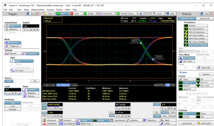
Figure 34. Disclosed 2.5 Gb/s eye diagram acquired with the FemtoScope 1051.
