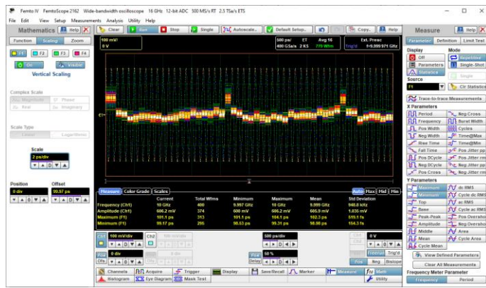
Figure 40. Trend of period measures nonlinearly of oscilloscope time base with 10-GHz sine wave. Maximum trend of period = 102.3 ps. Minimum trend of period = 98.98 ps. Peak-peak nonlinearity is within \pm 2.3 ps at 5 ns timing window.
