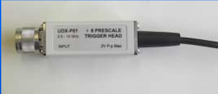
The UDX-P01 Trigger Head and its different options
