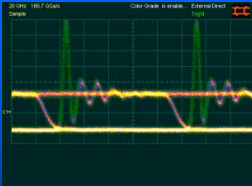
Waveform with No LP-Filtering
