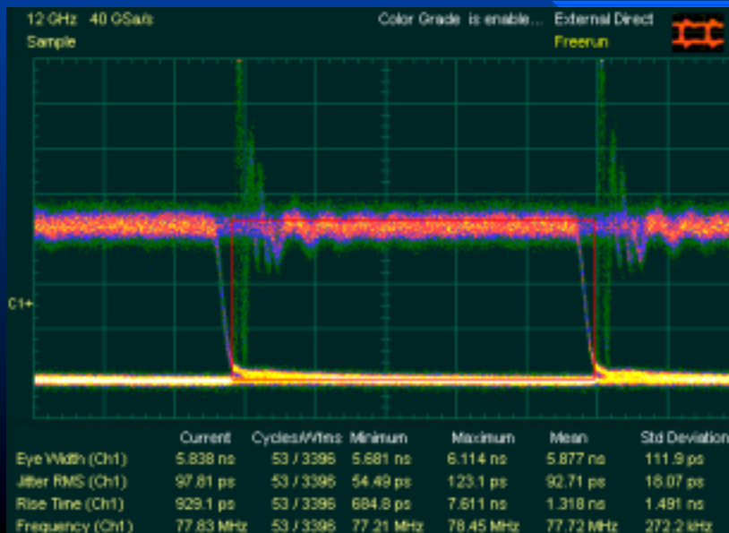
Noise measurement with No LP-Filtering
