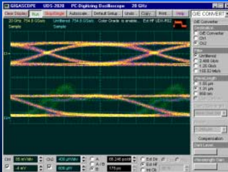
Top: 2.5-Gbps electrical eye-diagram. Bottom: 2.5-Gbps optical eye-diagram.
