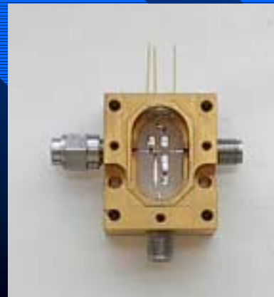
The UDS-2030 oscilloscope and a 30-GHz sampler
