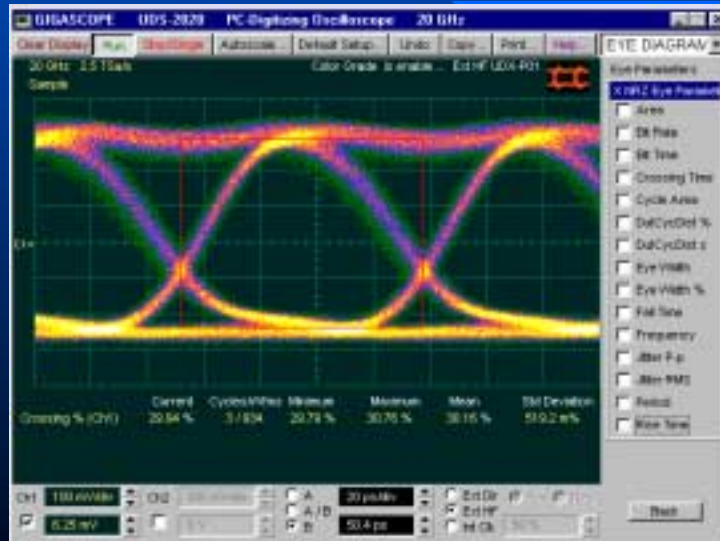
Crossing measurement of high-distorted 12-Gbit Eye Diagram
