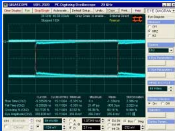
Timing measurements of 155-Mbit Eye Diagram
