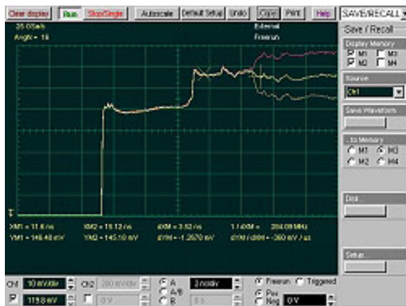
Figure 8. TDR of a 220-mm long PCB-pairline (no ground level). The coupling between the SMA connector (PCB I/O line) and pulse source made with 0.5-m RG-316 coaxial cable. The line is terminated with 120 Ohm (red), 75 Ohm (yellow) and 50 Ohm (green) resistors. Waveforms of the reflections show that the characteristic impedance Z_c of the line is equal to (85 \pm 3) Ohm. Inductive and capacitive discontinuities of the line and the connectors can clearly be seen.
