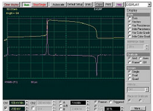
Figure 15. A signal's high-frequency content can be predicted with the order n of the spectral roll-off. In the figure above the signal (yellow) is differentiated once (violet) with large impulses as result.
