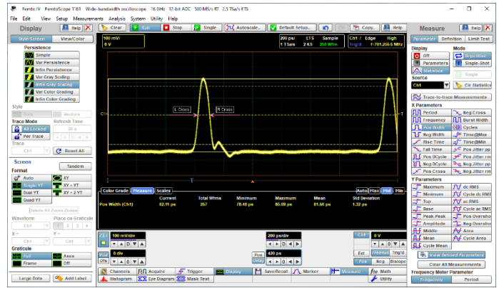
Figure 18. The FemtoScope 1161 demonstrates internal direct trigger from 81-ps pulse having 400 mV amplitude and 781 MHz frequency
