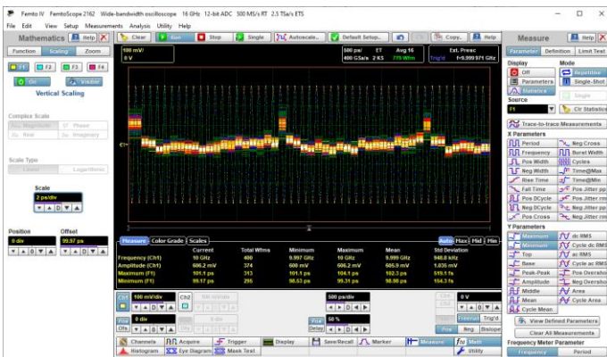
Figure 37. Trend of period measures nonlinearity of oscilloscope time base with 10-GHz sine wave (period 100 ps). Maximum trend of period = 102.3 ps. Minimum trend of period = 98.98 ps
