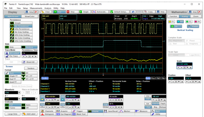
Figure 35. Example of algebraic functions (from top to bottom): a) channel 1 (data pattern), b) channel 2 (clock), c) integral of channel 1 d) differential of channel 1
