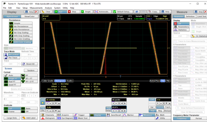
Figure 16. The FemtoScope 1051 surely triggers from 2.5 GHz sine wave with 1.62 ps rms jitter using internal trigger source
