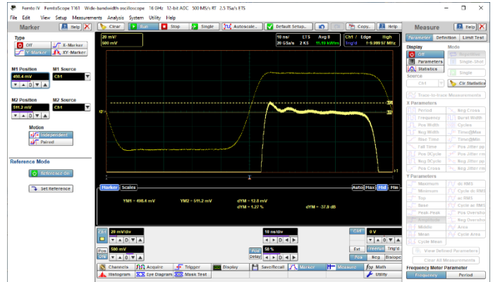
Figure 24. Ratiometric measurements. 1-V pulse is used as a reference. Two Y-markers measure 1.27% peak-peak ringing on the top of pulse
