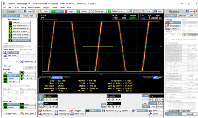
Figure 29. Horizontal histogram measures 1.64 ps rms jitter of 5-GHz sine wave (Std Deviation value)
