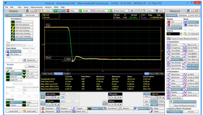
Figure 5. Transient response of the FemtoScope 2162 tested with Keysight N2806A Calibration Generator. Total measured fall time is 23.71 ps, rms jitter is 1.256 ps, and negative overshoot is 5.495%
