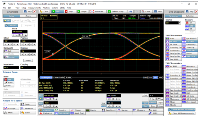
Figure 9. 800 Mb/s wide opened eye diagram acquired in narrow bandwidth mode shows good response characteristics
