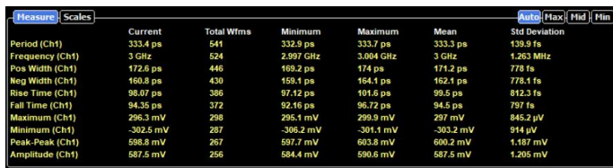
Figure 26. Snapshot tab with the results of ten measurements with full statistic
