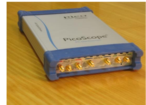
The PS9311: Dual-channel, 20 GHz with 55 ps rise time / 6 V TDR/TDT differential pulse generator
