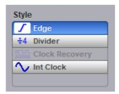
There are several different styles of trigger used in digitizing oscilloscopes. The PicoScope 9404 uses **Edge**, **Divided**, **Clock recovery**, **Internal clock** and **External Prescaler** styles.
