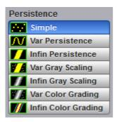
The **Persistence** menu determines how the data is displayed. There are seven choices for drawing waveforms:
