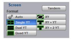
The **Format** menu determines how the instrument draws the waveforms on the display. The following formats are used in the PicoScope 9404.
