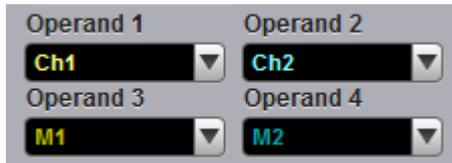
The instrument performs math functions on the source(s) (operands) you select. The math operator is performed either on operand 1, or on operand 1 and operand 2, or on operands 1 to 4. The number of operands used depends on the math operator you select. For example, **Add** requires two operands while **Invert** requires only one operand.
