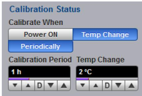
Choose when to calibrate the oscilloscope:
