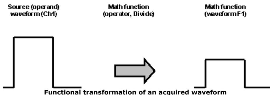
Create math waveforms to support the analysis of your channel and reference waveforms. By combining and transforming source waveforms and other data into math waveforms, you can derive the data view that your application requires.
