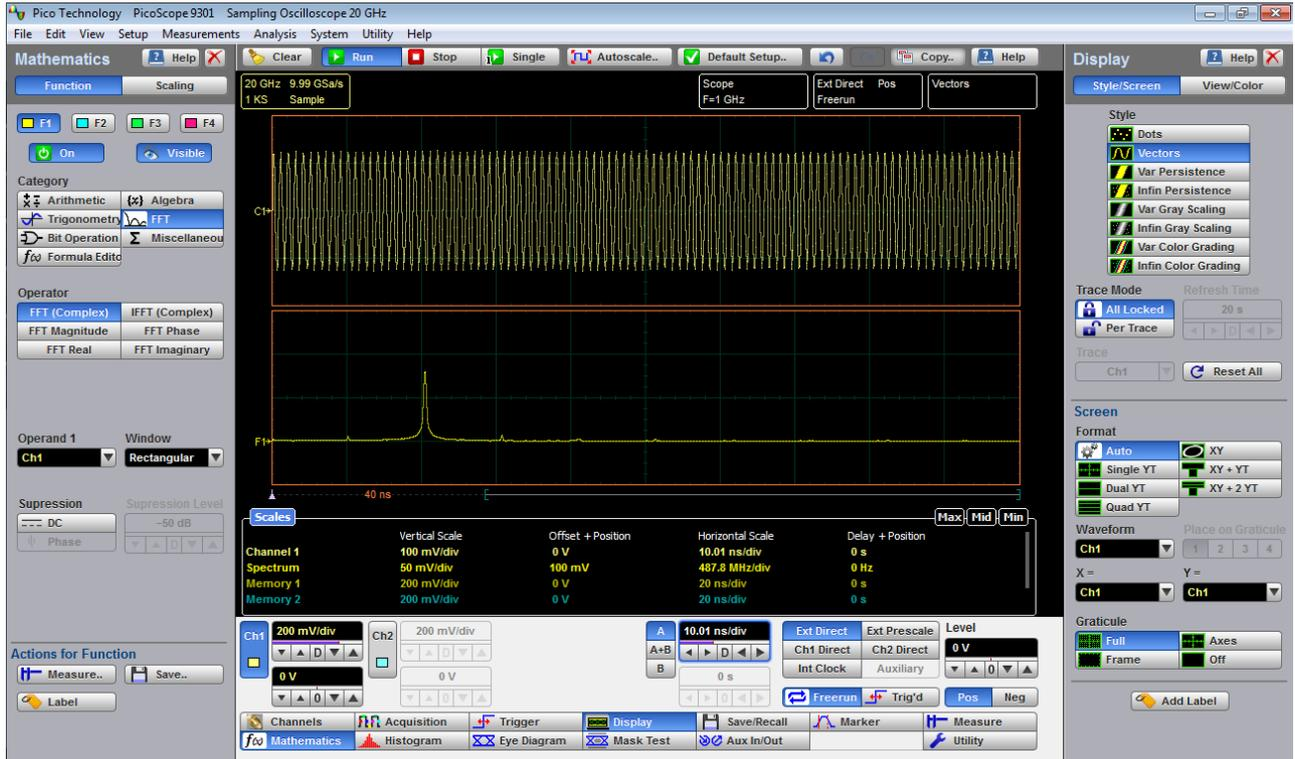
FFT with leakage
