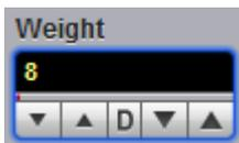
The **Weight** variable specifies the degree of influence of the latest acquired waveform against more remote waveforms. The **Weight** variable is active when **Exponential** is selected in the [Mode](#) menu. The **Weight** can be varied from 8 to 8192 in multiples of two.
