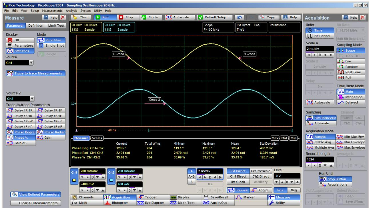
Example of phase measurement between two sine-wave waveforms
