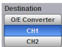
The **Destination** menu defines the optical configuration of the PicoScope 9321.
