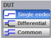
The DUT allows you to select between single-ended, differential or common TDR/TDT modes.
