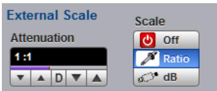
The **External Scale** functions can be used when the trigger signal level changes due to the use of an amplifier, attenuator or a probe. The attenuation factor can be entered either as a ratio or decibel value.
