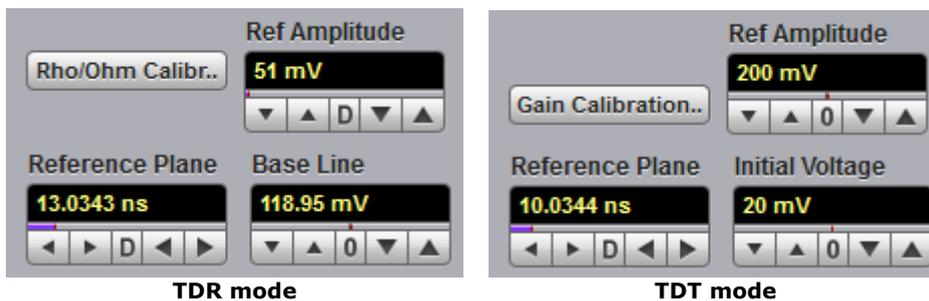
These controls allow you to calibrate the instrument for accurate **rho** and **ohm** measurements in **TDR** mode or accurate **gain** measurement in **TDT** mode.
