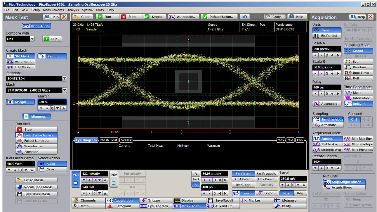
An example of eye-diagram with negative mask margins ( $-30\%$ )
