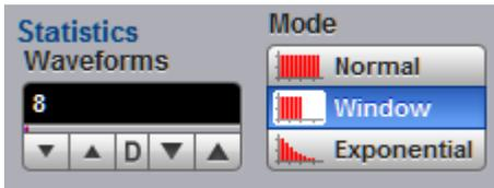
The **Statistics** menu includes modes and variables that determine the algorithm for a statistical measurement calculation. The **Statistics...** menu is active only when the **Statistics** mode of the **Display** menu is selected.
