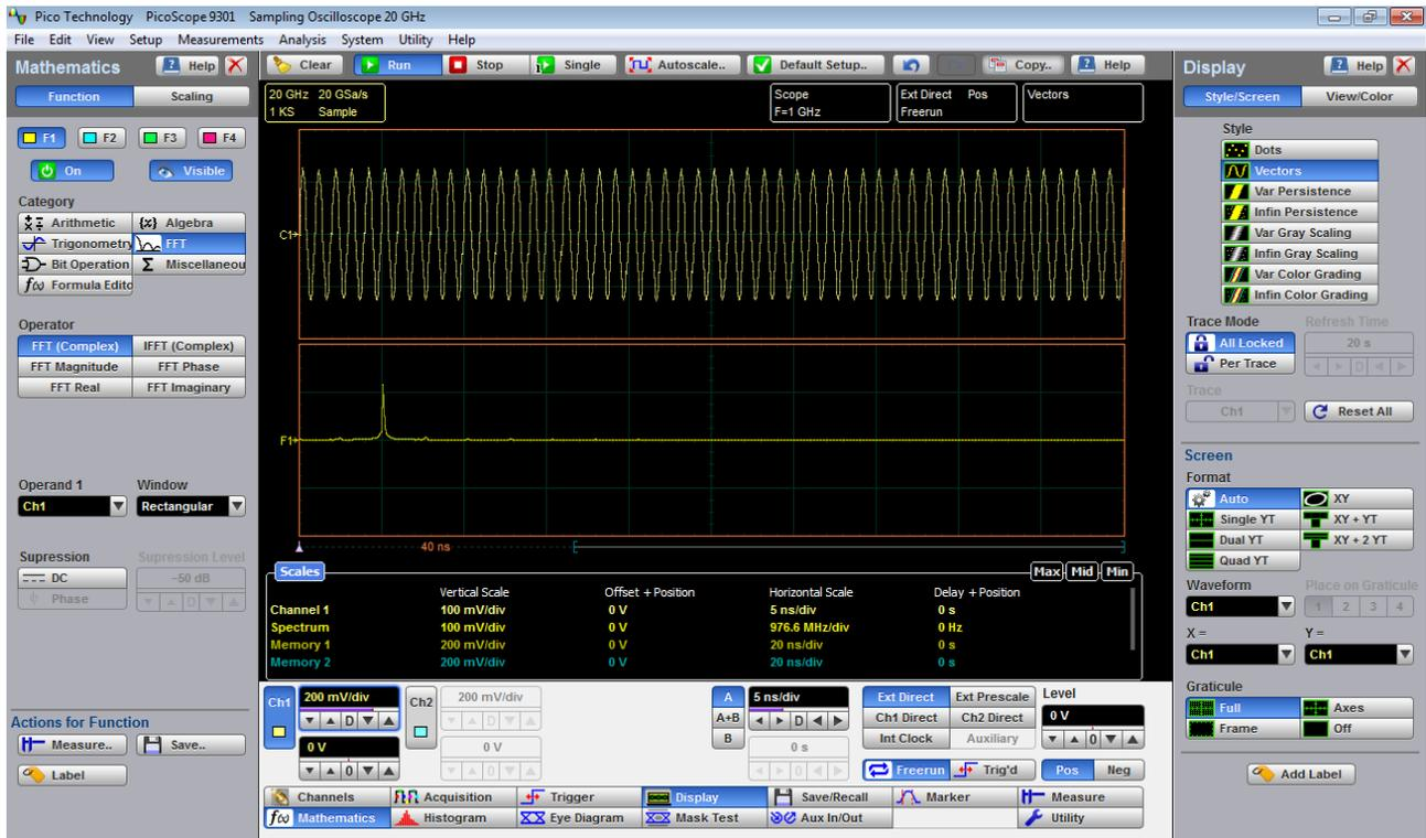
The 1 GHz sine-wave signal shown in both the Time Domain and the Frequency Domain
