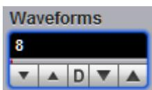
The **Waveforms** variable specifies the number of recently acquired waveforms used for statistical measurement calculations. The variable is active when **Window** is selected in the **Mode** menu. It can be varied from 8 to 8192 in multiples of two.
