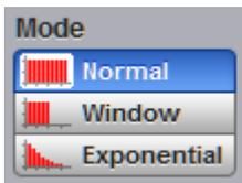
The Statistics **Mode** menu selects one of three modes that determine the algorithm for statistical measurement calculations.
