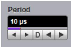
Pulse cycle time can be set as period. Period value can be set simultaneously for both outputs from 1  $\mu$ s to 60 ms, adjustable in 1-2-5-10 and 60 ms coarse increments. It is also adjustable in fine increments of 25 ns or 5 digits, whichever is greater.
