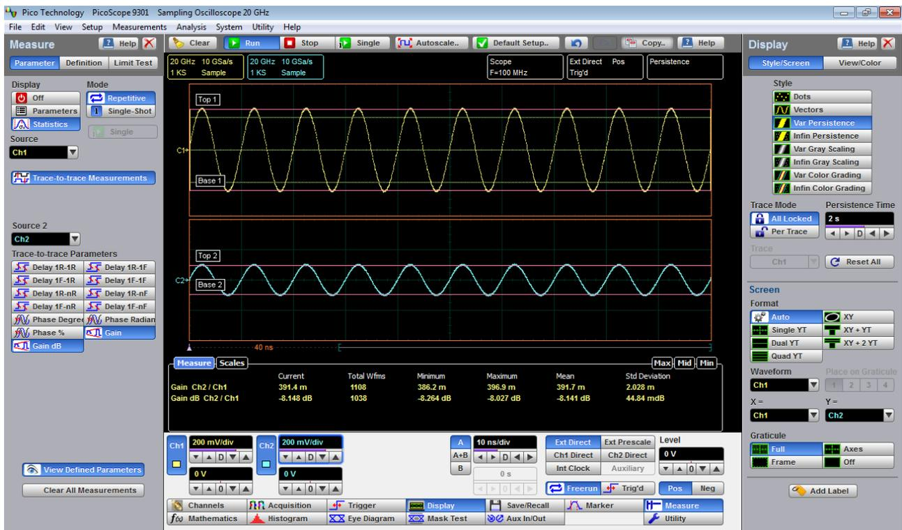
Example of gain measurement between two sine-wave signals
