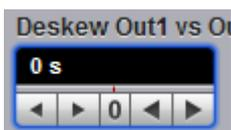
Set the deskew between **Positive Output** and **Negative Output** to compensate for different cable delays. Set the deskew outputs in typical range of -1.00 ns to 1.00 ns. Adjustable in a 20 ps coarse increment or in 1 ps fine increment.
