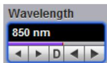
When an existing user-defined wavelength is selected from the [Calibration Point](#) list, the **Wavelength** control allows modification of the wavelength value.
