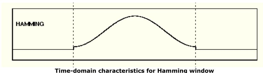
The **Hamming** window tapers the data to smaller values, but not to zero. It decreases the amount of energy spillover into adjacent frequency bins, increasing the amount of amplitude accuracy at the expense of decreasing the frequency.
