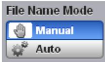
The **File Name Mode** control sets how the oscilloscope creates the name of the file. This control is enabled when the **File Type** control is set to **Waveform**:
