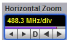
The **Horizontal Zoom** control allows you to zoom into a portion of the waveform record. Horizontal zooming can be entered in steps of 1-2-4-8. Changing the horizontal magnification of an FFT waveform using the **Horizontal Zoom** changes the appearance of the trace, but does not increase the horizontal (frequency) resolution.
