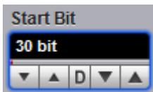
Set **Start Bit** to specify the starting bit location for the scan.
