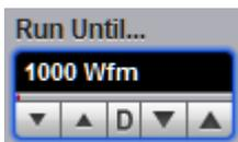
The **Run Until...** control is enabled when **File Type** is set to **Database**. It allows you to determine when the acquisition of the waveform database stops.
