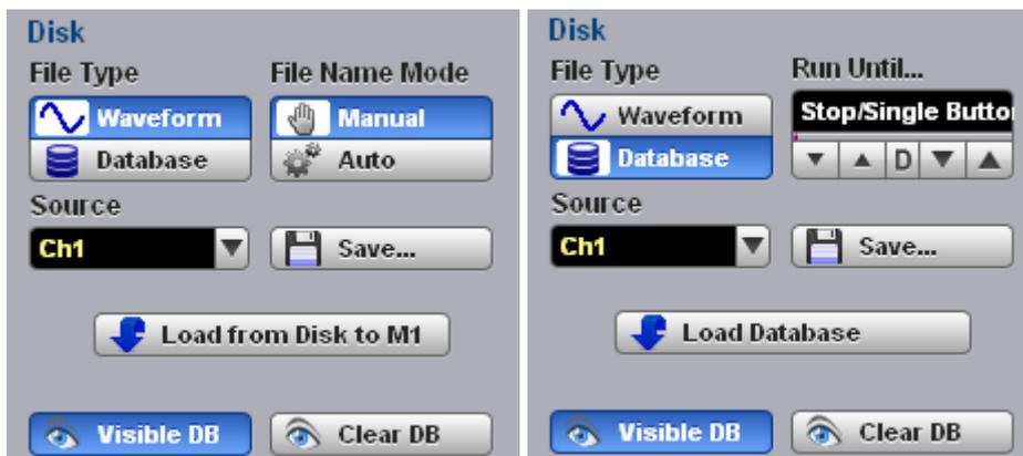
The **Disk** menu allows you to save your acquired waveform or database as an arbitrary file to disk. You can load these waveforms at a later time into the waveform memory (**M1 – M4**), and display them on the screen. Databases (**DB**) also can be loaded and displayed, but not via the waveform memory (**M1 – M4**).
