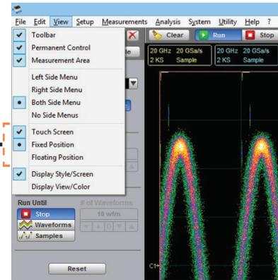
The image below shows PicoSample 3's touchscreen support in action: the box defining the histogram was drawn by hand, and the enlarged parameter control is being used to control the Channel 1 voltage scale.
