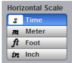
The **Horizontal Scale** menu selects one of the horizontal units of measure commonly used in TDR/TDT.
