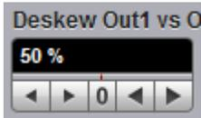
Set the deskew between **Positive Output** and **Negative Output** to compensate for different cable delays. Set the deskew outputs in typical range of  $-500$  ps to  $500$  ps. Adjustable in  $20$  ps coarse increments or  $1$  ps fine increments.
