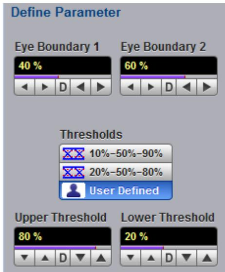
The **Define Parameters** menu sets the measurement points (boundaries and thresholds) where the automatic measurements are made. The menu influences the measurement algorithm by allowing you to use the standard measurement points, or customize the measurements with user-defined selections.
