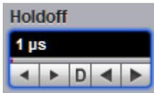
Trigger **holdoff** helps stabilize [triggering](#). When you adjust the **Holdoff** control, the amount of time that the scope waits before re-arming the trigger circuitry also changes.
