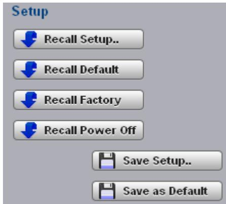
To save a current setup for later use, you can use any drive available to the PicoScope 9300's PC. When you save a setup, all of PicoScope 9300's settings, including measurements, markers, horizontal and vertical control settings, trigger configuration, color scheme, and math functions, are saved.
