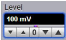
The **Level** variable specifies the voltage threshold that a signal must cross in order for the instrument to trigger on that signal. When the input signal crosses this voltage level, the instrument triggers.
