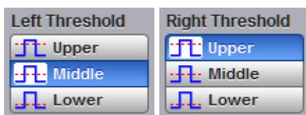
The **Left Threshold** and **Right Threshold** variables select crossing points on the edge of the selected waveform. Both variables can be used only when **Waveform** is selected in the **Mode** menu.
