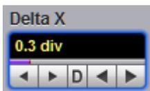
The **Delta X** variable defines the horizontal tolerance around the edges of the reference waveform.
