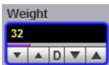
The **Weight** variable specifies the degree of influence of the nearest acquired waveform against more remote waveforms. The **Weight** variable is active when **Exponential** is selected in the **Mode** menu. The **Weight** can be varied from 8 to 8192 in multiples of two.
