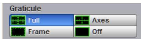
The PicoScope 9300 Series has a 10 by 8 display graticule grid, which you can turn on or off. The **Graticule** menu selection is:
