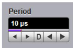
**Period** sets the pulse cycle time. The value can be set simultaneously for both outputs from 1 μs to 60 ms. Adjustable in 1-2-5-10 and 60 ms coarse increment. Also adjustable in fine increments of 25 ns or 5 digits, whichever is greater.
