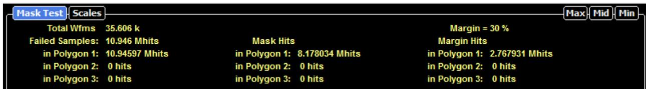
Measurement Area of Mask Test
