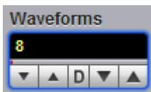
The **Waveforms** variable specifies the number of influenced waveforms when the **Window** is selected in the [Mode](#) menu. The **Waveforms** can be varied from 8 to 8192 in multiples of two.
