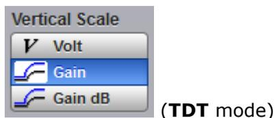
In addition to the voltage scale, **TDT** can also use **Gain** scaling.
