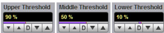
The **Upper Threshold**, **Middle Threshold**, and **Lower Threshold** variables are displayed only when **User Defined** is selected in the [Thresholds](#) menu. All variables can be selected for either **Percent**, **Volt** (or **Watts**), or **Division**.
