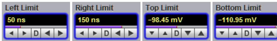
The **Left Limit**, **Right Limit**, **Top Limit** and **Bottom Limit variables** allow you to use the histogram limits to select a region of the database.
