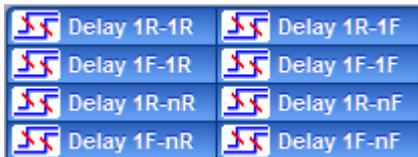
**Delay** is defined as the time interval between the crossings of the two mid-reference levels on the two sources of the measurement. The PicoScope 9300 starts the measurement on the first edge on the leftmost portion of the measurement region (left margin) and stops the measurement on the last edge on the rightmost portion of the measurement region (right margin).
