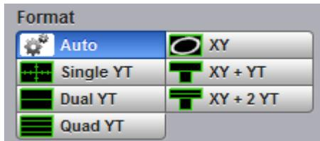
The **Format** menu determines how the instrument draws the waveforms on the display. The following formats are used in the PicoScope 9300 Series.
