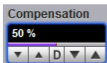
The **Compensation** control shows the result of dark-level calibration. It may also be used for manual control of dark level.
