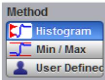
The **Method** menu sets the **Top** and **Base** vertical reference thresholds for amplitude measurements. It also sets the values from which the upper, middle and lower thresholds are calculated. The **Top** and **Base** variables are displayed when the **User Defined** method is selected. The three selections under the **Method** menu allow the user to choose the method for determining the **Top** and **Base** of the waveform.
