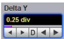
The **Delta Y** variable defines the vertical tolerance around the edges of the reference waveform.
