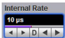
The **Internal Rate** spin-box allows you to vary the repetition rate of the internal clock from 8 ns to 60 ms. If fine mode is off, the repetition rate can be set in a 1-2-5 sequence. When fine mode is on, you can change the repetition rate in 4 ns increments.
