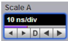
The **Scale A** function is similar to the time/div knob of the main timebase on a traditional oscilloscope. *Division* in this instance equals 1/10 of the horizontal axis. Adjusting the horizontal (timebase) scale control expands and compresses the displayed waveform horizontally.
