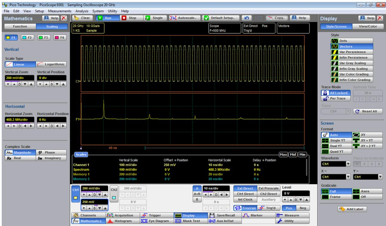
**Spectrum Magnitude of 500 MHz pulse waveform**
