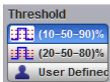
The **Threshold** control sets the measurement points that the automatic measurements use for calculating the timing measurement results. The threshold points are upper, middle, and lower. For example, rise time is measured from the lower threshold to the upper threshold, while a width measurement is made between two middle thresholds.
