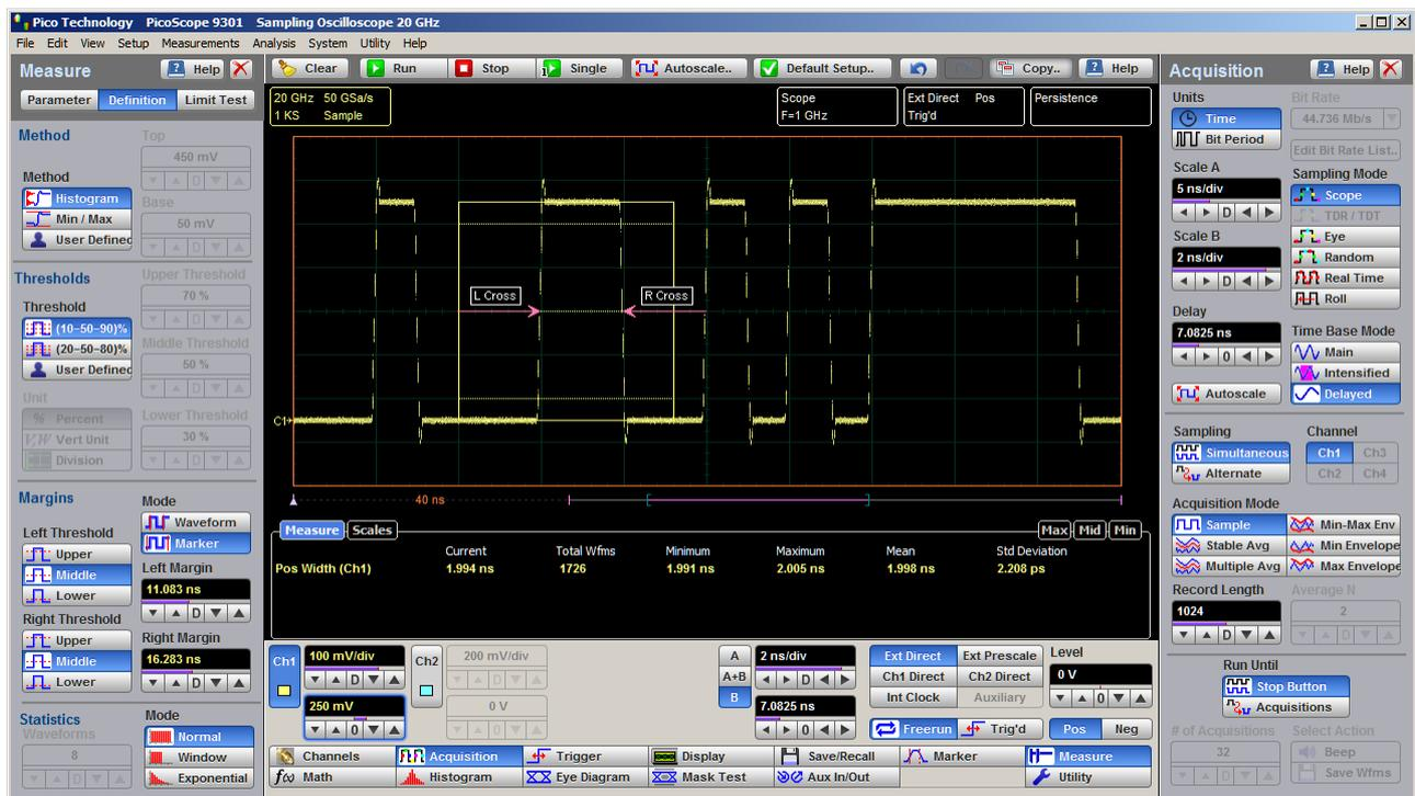
Correct position of both margins provides width measurement of second short pulse
