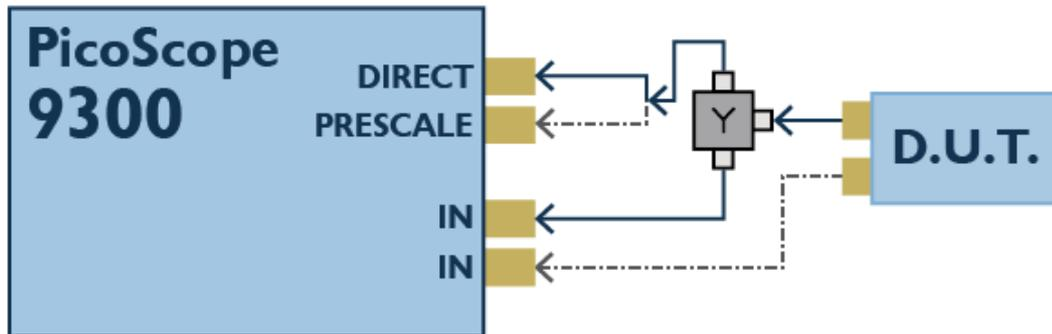
Basic setup for all 9300 Series PicoScopes
