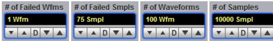
When **Failed Waveforms** in the **Run Until** menu is selected, the **# of Failed Wfms** variable sets the number of failed waveforms. After this number is reached, acquisition stops.
