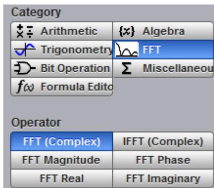
The **FFT** menu allows you to control the operation of the FFT (Fast Fourier Transform), including spectrum selection and display, and also a choice of six FFT windowing functions. Refer to the **Scaling** menu for formatting a spectrum with different complex scales, and also for scaling and positioning it.
