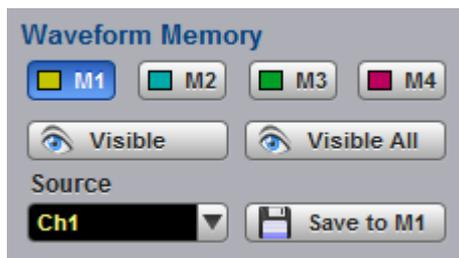
The instrument allows you to save your acquired waveforms to any of the instrument's internal drives. You can recall these waveforms at a later time and display them on the instrument's display screen. The **Waveform Memory** menu allows you to save or recall a waveform into one of the waveform memories (**M1 – M4**), intended for display.
