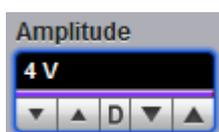
Amplitude is the low-to-high magnitude of the pulse. The **Amplitude** setting changes from 2.5 V to 6 V. Adjustable in a 100 mV coarse increment or in 5 mV fine increment. Changing the amplitude will change the high level only. Low level is always at 0 V. Offset is not affected.
