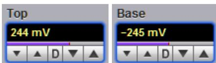
The **Top** and **Base** variables let you set the top and base to a specific voltage value. As an example, for a 200 mV/div vertical scale you can set the top and base voltage values from -798 mV to 798 mV in 25 mV (coarse) or 1.56 mV (fine) increments determined by the voltage range you are in.
