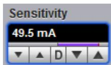
**Sensitivity** controls the peak current of TD manually when the **Manual** is selected from the **TD Current**.
