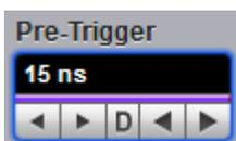
The output pre-trigger signal on the **TRIGGER OUTPUT** connector marks the start of the pulse period. This positive pulse has fixed near 700 mV amplitude, 25 ns to 35 ns lead-time range adjustable in 100 ps coarse increments or 5 ps fine increments.
