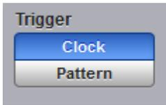
In PRBS mode, the scope can be set to trigger on either the data **Clock** or the **Pattern** detector.
