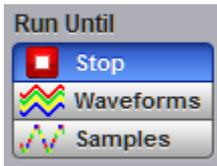
The **Run Until** menu allows you to determine when the acquisition of data stops.
