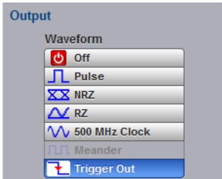
**Trigger Out** mode allows you to select a pulse waveform synchronous to internal holdoff trigger and internal TDR clock. Negative transient is active.
