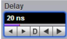
In one of **Sequential Equivalent Time Sampling Modes** (**Scope**, **TDR/TDT** or **Eye**) the **Delay** function is similar to the delay knob of the delayed timebase on a traditional oscilloscope. The **Delay** spin-box allows you to the position of delayed timebase up to maximum value of 10 divisions of main timebase in one of three ways:
