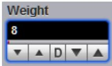
The **Weight** variable specifies the degree of influence of each recently acquired waveform against more remote waveforms. The variable is active when **Exponential** is selected in the **Mode** menu. **Weight** can be varied from 8 to 8192 in multiples of two.
