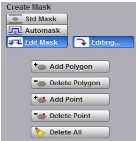
The **Edit Mask** function gives you access to a menu that allows you to construct a new mask, or edit an existing one, using the polygon method. The procedure of editing a mask function brings up a set of brief instructions on how to construct a mask.
