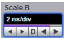
The **Scale B** function is similar to the time/div knob of the delayed timebase on a traditional oscilloscope. Adjusting the delayed timebase scale control expands and compresses the displayed waveform horizontally.
