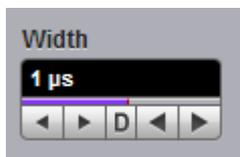
**Width** is the absolute pulse width measured from the start of the leading edge to the start of the trailing edge. In this format, the pulse width is independent of changes in pulse period and delay. Pulse width is defined at the 50% amplitude level of the pulse.
