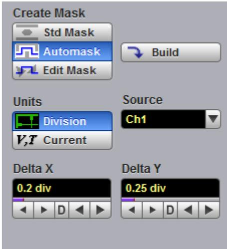
Clicking the **Automask** opens a menu for using the reference waveform method. An example of the method for a noisy impulse is shown in the figure below.
