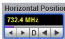
The **Horizontal Position** control allows you to move the horizontally expanded portion of the waveform record. The **Horizontal Position** variable uses software positioning.
