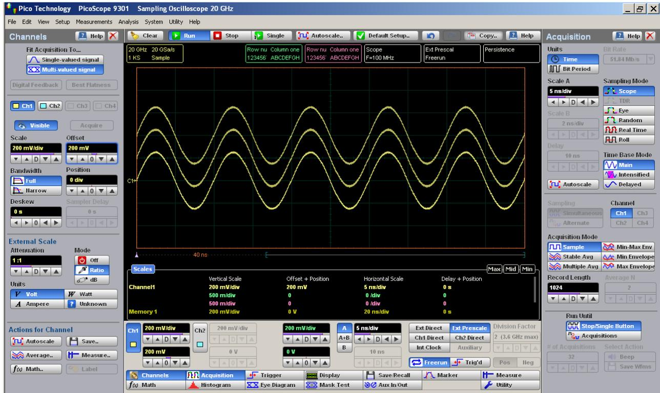
Sine-wave signal with different offsets
