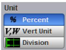
You can set the unit of measure for upper, middle, and lower thresholds to **Percent**, **Vertical Unit** or **Division**.
