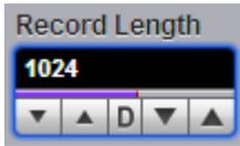
The number of samples that form a trace is called the record length. For example, if the horizontal (timebase) scale is set up as 10 ns/div, the total displayed sweep time is 100 ns. The more sampled data that is available for analysis or measurements, the greater the record length.
