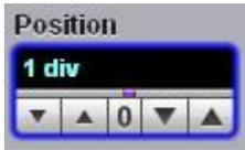
Use the **Position** variable to set the vertical position of the selected channel on the display without changing its offset value. The visual effect is the same as for **Offset** but the waveform is adjusted at a later time in the signal flow.
