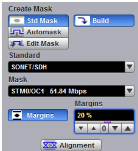
Clicking the **Std Mask** allows you to select from a variety of standard telecommunication masks.
