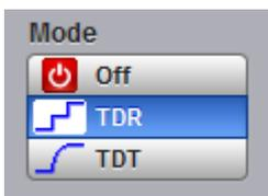
The **Mode** menu lets you control the TDR/TDT functions of the PicoScope 9311/9312. The selector turns the features to **Off**, or enables **TDR** or **TDT**. When you switch the instrument to **TDR** or **TDT** mode the acquisition system automatically switches into **Single-valued signal** acquisition with stable averaging and averaging.
