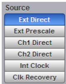
The **Source** menu specifies the signal that the trigger system monitors. The **Source** function displays a list of the available trigger sources. There are six sources that the PicoScope 9300 can use for a trigger:
