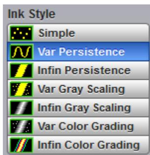
The **Ink Style** menu determines how the data is displayed. There are seven choices for drawing waveforms:
