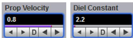
The **Propagation Velocity** or **Dielectric Constant** controls let you specify the fraction of the speed of light at which the signal passes through your transmission line or network. Both controls apply only to axis units of distance, and do not apply if your horizontal units are seconds.
