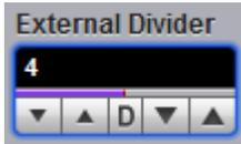
Select **Auto** in the **Pattern Lock** menu to have the trigger divide ratio automatically detected. You can also manually enter the trigger divide ratio.
