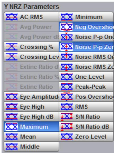
The list of **Y NRZ Eye Parameters** includes twenty-seven eye parameters. Two of the them (**Avg Power** and **Avg Power dBm**) can be used in optical models only.
