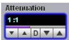
The **Attenuation** variable lets you select an attenuation that matches the device connected to the instrument. When the attenuation is set correctly, the instrument maintains the current scale factors if possible. All marker values and voltage, amperage or wattage measurements will reflect the actual signal at the input to the external device.
