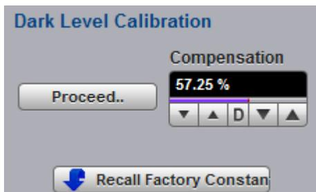
The **Dark Level Calibration** menu provides a dark-level calibration that maximize the accuracy of the extinction ratio and other optical automatic measurements you take.
