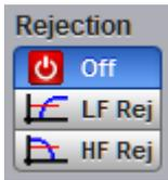
The trigger rejection determines which frequency components of the signal are passed to the trigger circuitry. This function is available with the **Ch1 Direct** and **Ch2 Direct Trigger Sources** only.
