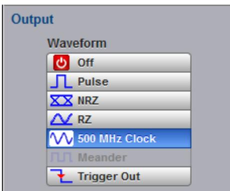
**500 MHz Clock** output mode allows you to select a 500 MHz waveform close to a sinusoidal clock. This clock is synchronous to the internal clock.
