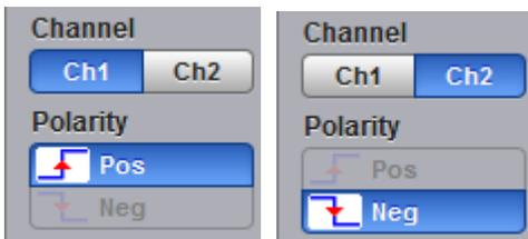
The **Channel** menu assigns the function keys to the selected channel. You can assign the **Vertical Scale**, **Ref Amplitude** and **Base Line** (TDR mode) or **Initial Voltage** (TDT mode) for selected channel.
