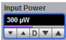
The **Input Power** control shows the calibration source power.
