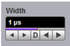
The absolute pulse width measured from the start of the leading edge to the start of the trailing edge. In this format, the pulse width is independent of changes in pulse period and delay. Pulse width is defined at the 50% amplitude level of the pulse.
