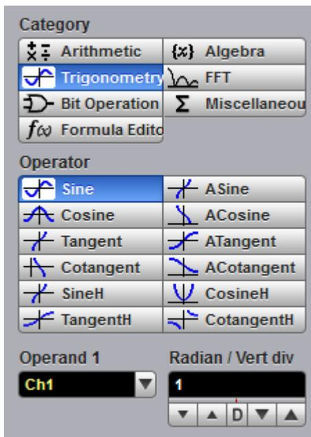
Below is a description of the twelve trigonometric operators. There are four standard trigonometric functions, four inverse trigonometric functions, and four hyperbolic functions.
