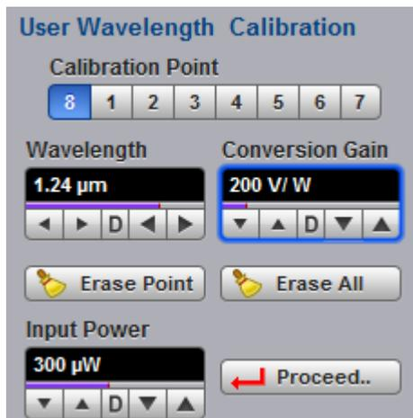
The **User Wavelength Calibration** menu allows optical channel calibration for user-defined wavelengths. You can set any wavelength between 750 nm and 1650 nm.
