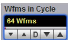
The **Wfms in Cycle** variable determines how many acquired waveforms will be used for the one-measurement cycle in eye diagram calculations.
