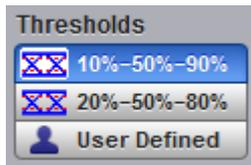
The **Thresholds** menu sets the upper, middle, and lower measurement points that the eye diagram measurements use for calculating the timing measurement results. For example, rise time is measured from the lower threshold to the upper threshold, while a RZ Pulse Width measurement is made between two middle thresholds.
