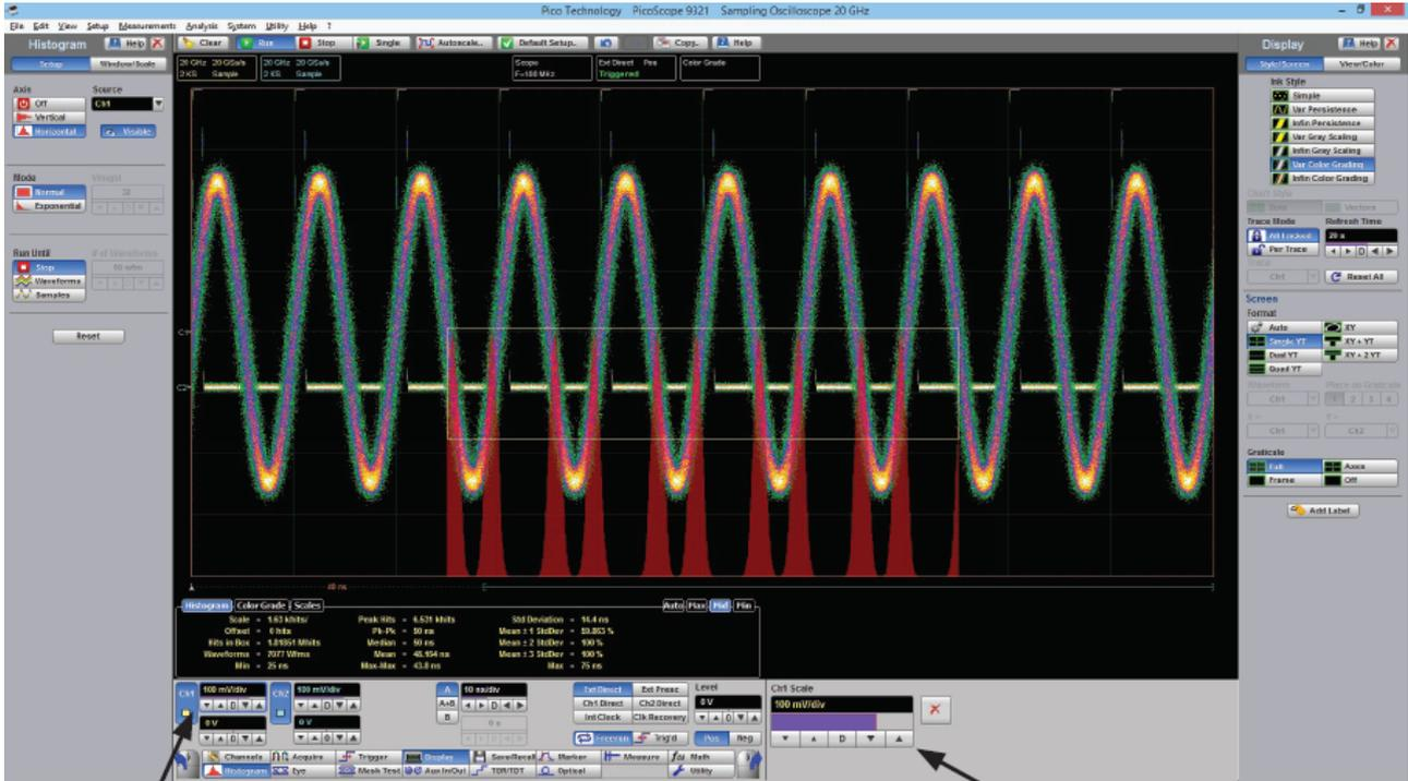
The Channel 1 voltage scale control is active (and highlighted in blue), but the buttons and the parameter overview bar are too small for easy use with the touch screen.
