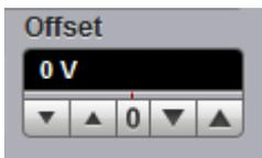
The DC offset of the signal. This is the mean voltage of a Sine signal, or the base voltage of a Pulse or PRBS signal.
