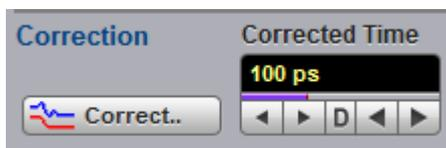
The **Correction** menu allows you to change the rise time of the corrected step for TDR or TDT measurements on each of the channels, and also to turn on or off the display of the corrected TDR or TDT trace (function).
