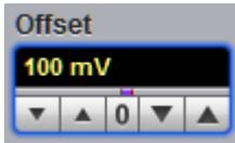
You can use the vertical **Offset** controls to move your waveform either up or down on the display. The **Offset** variable changes the vertical position of a particular channel's waveform on the display screen without modifying the waveform itself. It determines the portion of the input signal presented to the acquisition system.
