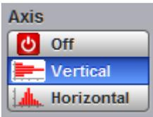
The **Axis** function turns the display of the histogram off or orients the histogram vertically or horizontally.
