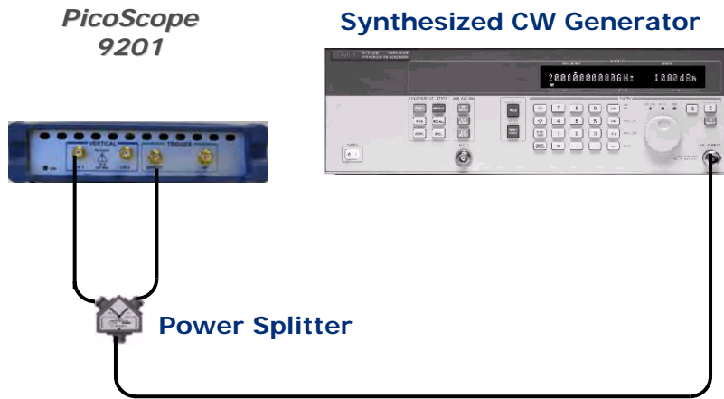
Equipment connections for Direct Trigger Test
