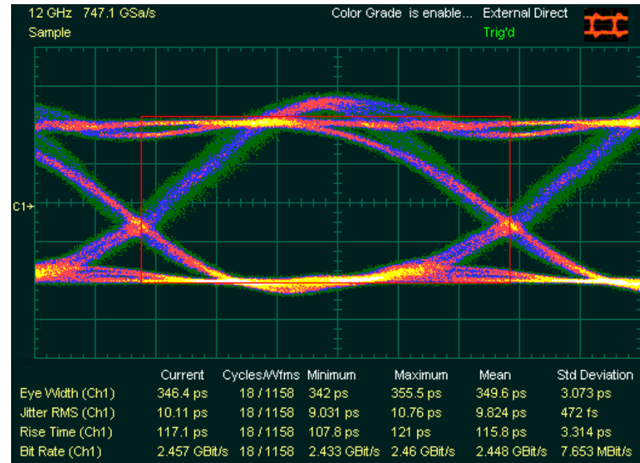
Eye-Diagram Measurements without (left) and with LP-Filtering.
