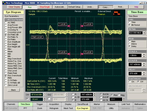
Measurement of 1.25-Gbit eye diagram
