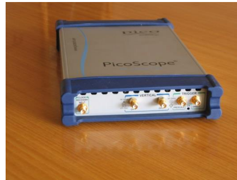
The PS9301: Dual-channel, 20 GHz with 11.3 Gbps clock recovery trigger
