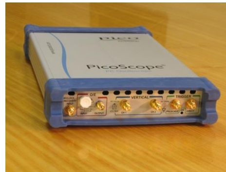
The PS9311: Dual-channel, 20 GHz with 9 GHz optical bandwidth and 11.3 Gbps clock recovery trigger
