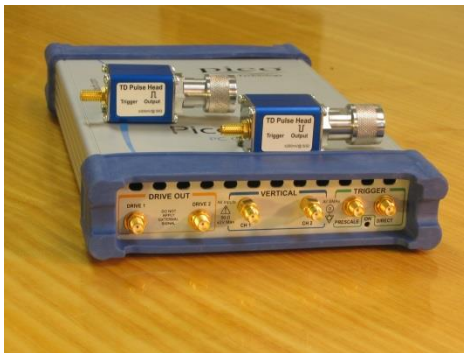
The PS9312: Dual-channel, 20 GHz with 35 ps rise time/200 mV TDR/TDT differential pulse generator
