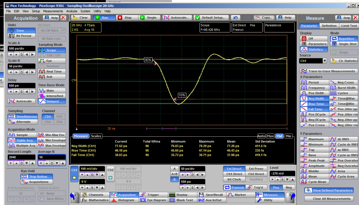
77-ps pulse acquired with Tektronix PPG1251 Pattern Generator
