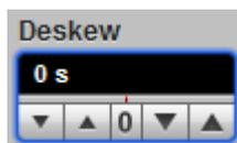
Set the deskew between **Positive Output** and **Negative Output** to compensate for different cable delays. Set the **Deskew** between output in the range of -1.00 ns to 1.00 ns. Adjustable in a 20 ps coarse increment or in 1 ps fine increment.
