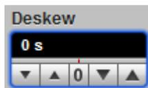
Set the deskew between **TD Head 1 Output** and **TD Head 2 Output** to compensate for different cable delays. Set the **Deskew** between output in the range of 0 ps to 500 ns. Adjustable in a 20 ps coarse increment or in 1 ps fine increment.
