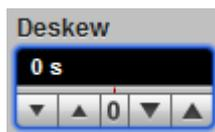
Set the deskew between **TD Head 1 Output** and **TD Head 2 Output** to compensate for different cable delays. Set the **Deskew** between output in the range of 0 ps to 500 ps. Adjustable in 20 ps coarse increments or in 1 ps fine increments.
