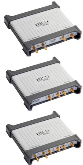
PicoSource Pulse Generators are capable of producing pulses of either polarity with very fast rise times. The generators will free-run or may be triggered from an external source, with either positive or negative pulses, at rates of up to 1 MHz. The units are designed to operate into 50  $\Omega$  lines.
