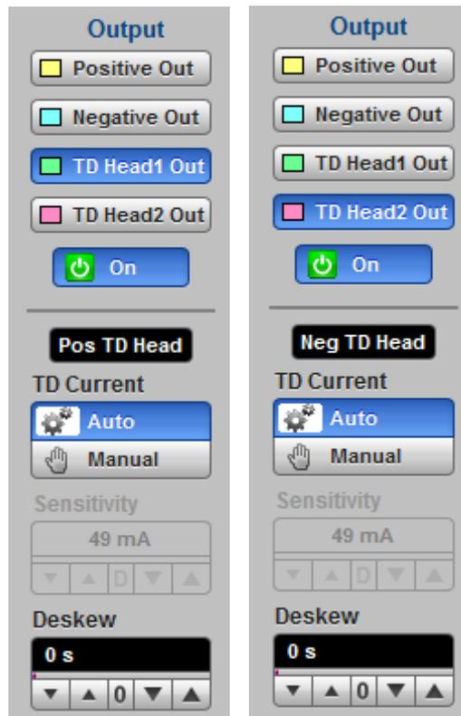
**TD Head 1 Output (left) and TD 2 Head Output (right) menus**
