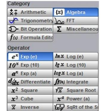
The PicoScope 9400 Series scopes support up to four simultaneous mathematical combinations or functional transformations of acquired waveforms.
