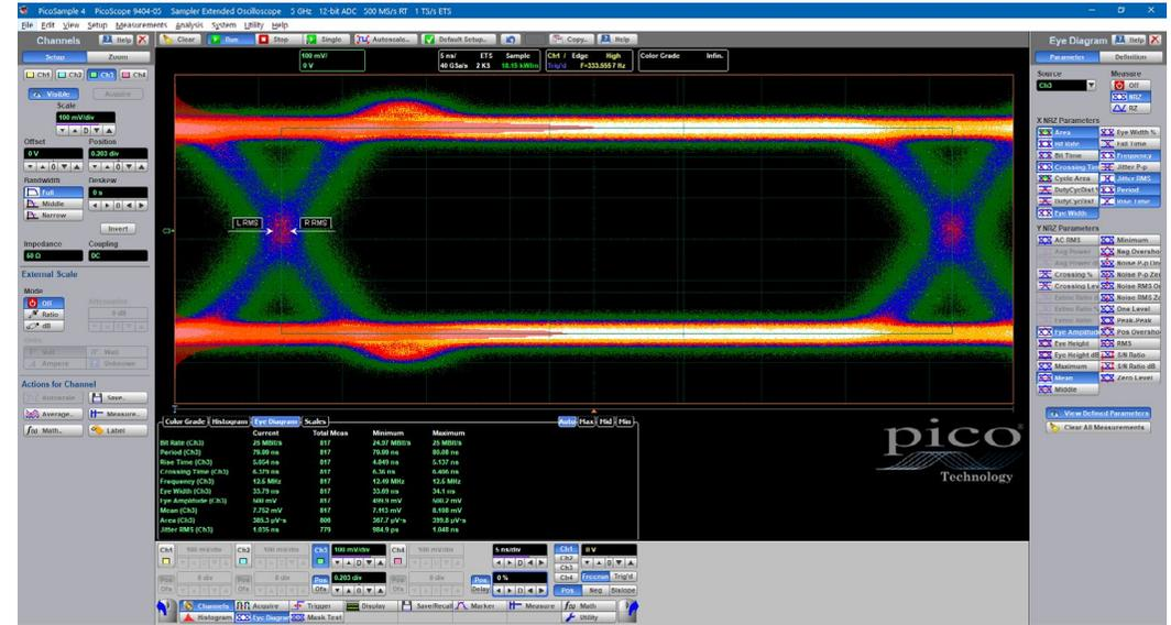
Eye-diagram analysis can be made even more powerful with the addition of mask testing, as described below.
