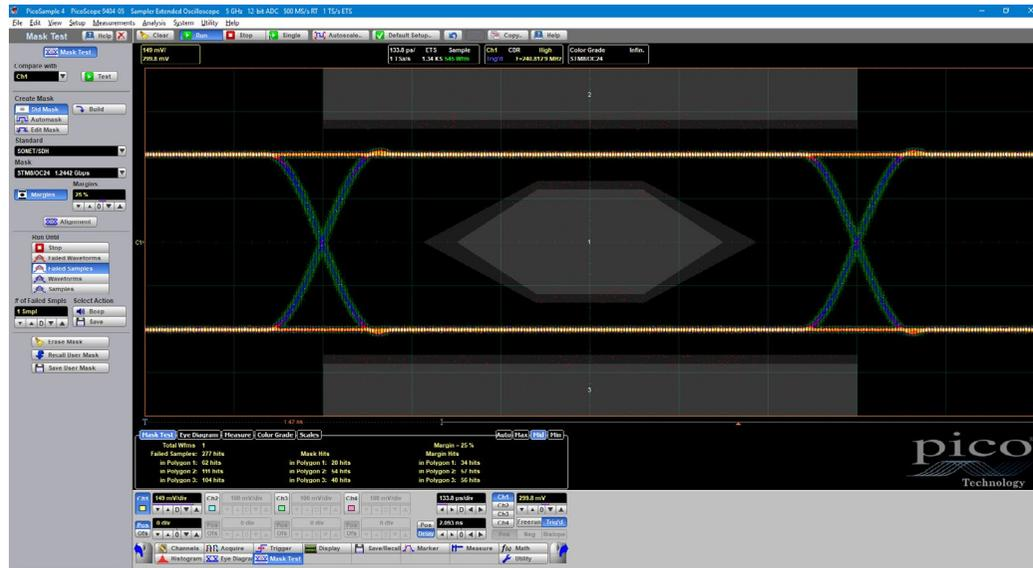
PicoSample 4 has a built-in library of over 130 masks for testing data eyes. It can count or capture mask hits or route them to an alarm or acquisition control. You can stress-test against a mask using a specified margin, and locally compile or edit masks.
