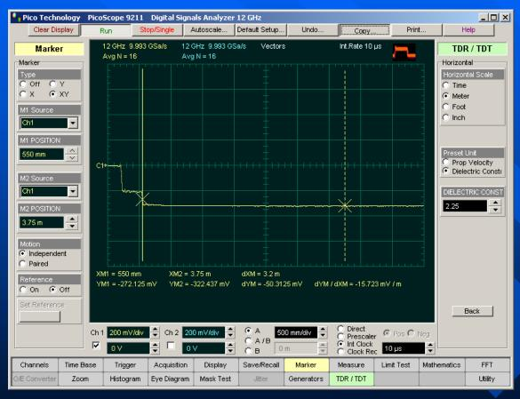
A TDR step can also be used to make Time Domain Transmission (TDT) measurements. TDT is a technique that allows you to measure the response of a system by sending steps through a device and monitoring the output of the device.
