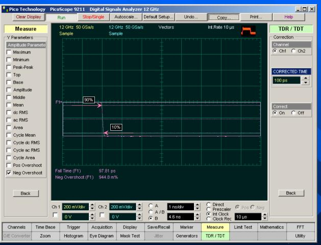
The Correction allows you to change the rise time of the corrected step for TDR or for TDT on each of the channels, and also to turn on or off the display of the normalized TDR or TDT trace (function).
