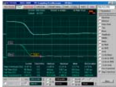
TDR Normalization. The top waveform shows distortions caused by cables and connectors. The bottom waveform shows how normalization corrects for these distortions.
