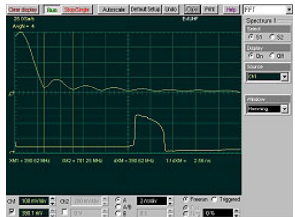
Figure 3. The magnitude of continuous Sinx/x-type spectrum of the pulse. 1/T_w = 390.62 MHz, 2/T_w = 781.25 MHz, Measured T_w (Pulse Width) = 2.56 ns
