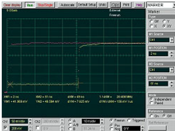
Figure 6. Pulse delay in a 9.6-m long 50-ohm coaxial cable (RG-213 type) is 49 ns. Propagation speed is 5.1 ns/m
