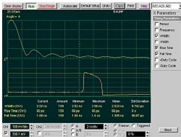
Figure 2. Pulse Width = 2.523 ns, Rise Time = 80 ps (10%-90%), Fall Time = 1.3 ns (10%-90%)
