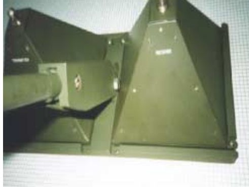
Figure 5: The antenna of the ITL231A Mine Detector covers the bandwidth 0.4 to 2.4 GHz and works with both 1 and 2 GHz central frequencies
