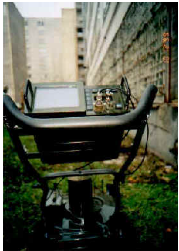
Figure 4: The ER2-02 Ground Penetrating Radar is a field-rugged impulse radar system designed for detection of features or objects buried within horizontal or vertical surface
